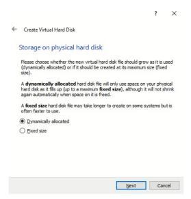
Select the desired location and size for the virtual hard disk. If a dynamic allocation method was selected in the previous step, this setting will be used to limit the maximum size of the virtual drive (allocation will take place as needed up to the selected size). If a fixed size was selected, the size entered here will be immediately reserved on the physical drive. The minimum recommended size is 20 GB.
