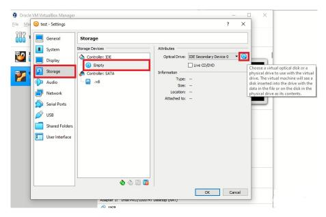
The Storage dialog should now show that the Ubuntu image is loaded into the IDE controller's virtual disk drive. Click ok to close the settings dialog.
