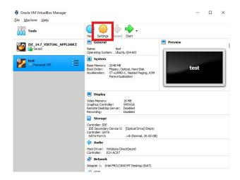
Use the settings menu to select Storage from the left hand menu. Next, select the currently empty device under the IDE controller. Then, click the CD icon and click the option to choose a disk file to select a disk which will be loaded into the virtual drive. Use the file browser dialog to select the Ubuntu 20.04 Desktop image that was downloaded earlier.
