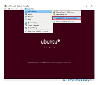
Upon rebooting, the login screen with the configured user name should appear. If the Ubuntu installation menu appears again, it will need to be removed manually through the settings dialog. Shutdown the machine. Using the menu select Machine then ACPI Shutdown.
