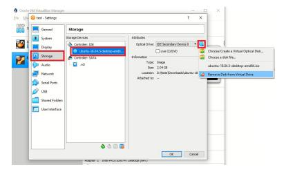
Now that the disk has been removed, close the settings dialog and start the virtual machine again.
