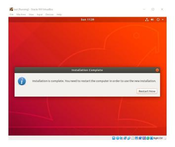
At this point, the installer will pause to give the user time to remove the installation disk. VirtualBox usually handles this automatically, but to verify the Ubuntu disk has been removed, click Devices then Optical Devices and ensure there is no check mark next to the Ubuntu disk image. If there is a check mark, click the disk image menu option and select force unmount. Hit the enter key to reboot the machine.
