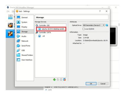
The virtual machine can now be powered on. Click the start button.
