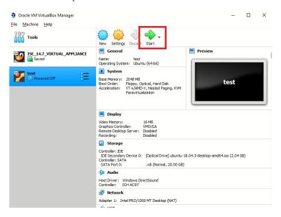
The virtual machine will start up and boot from the selected Ubuntu Desktop image found in the virtual disk drive. Click the Install Ubuntu button.
